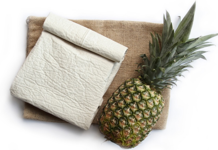
Pinatex Waste material of pineapples and used as a leather substitute. A multi-purpose material. Naomi Atmopawiro, Pezy Group
