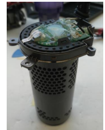
Example of bundling: both PCB and motor are electronics parts. But in this case, they are glued together.
